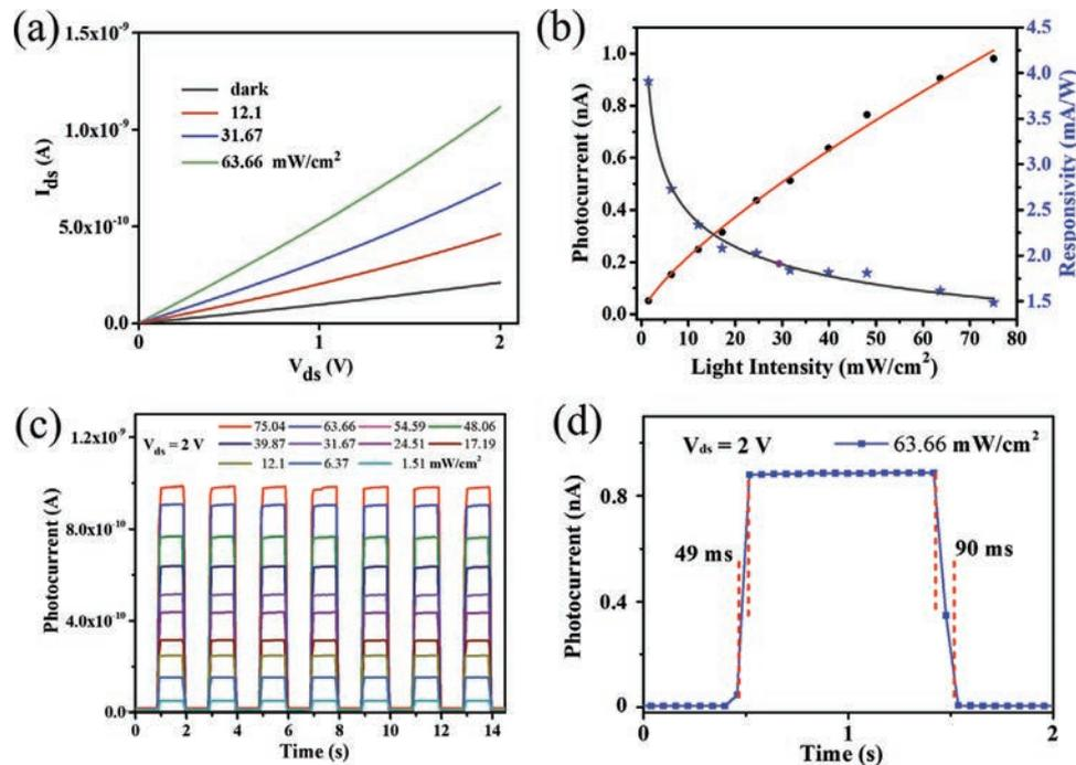
**Figure 5.** Photoresponse properties of the vdW PdSe<sub>2</sub>/WS<sub>2</sub> heterostructure photodetector towards 635 nm excitation. a) Photocurrent versus  $V_{ds}$  curves under illumination of different light power density. b) Photocurrent and responsivity versus power density. c) Photoresponse under different power density. d) High-resolution photocurrent versus time curve.
