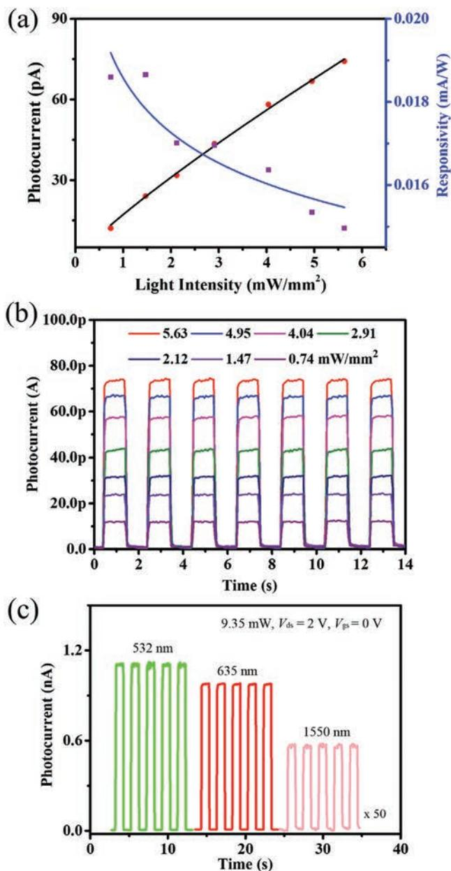
**Figure 6.** Broadband photoresponse properties of the vdW PdSe<sub>2</sub>/WS<sub>2</sub> heterostructure photodetector. a) Photocurrent and responsivity versus light power density at 1550 nm. b) Photoresponse under different power density at 1550 nm. c) Photoresponse under different light illumination wavelengths (532, 635, and 1550 nm), at a constant light power of 9.35 mW (light intensity: 74.0 mW cm<sup>-2</sup>).
