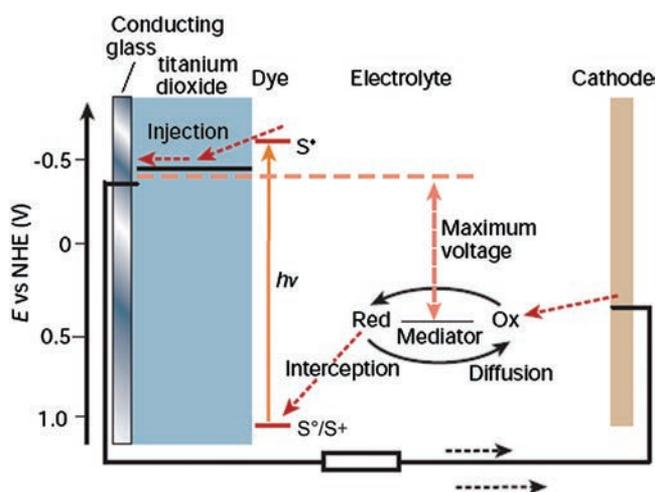
**Figure 6.** Mechanism of dye-sensitised solar cells. The titanium oxide photoanode receives electrons from photoexcited dyes. The positively charged dyes are then reduced by a mediator redox pair dissolved in the electrolyte. The mediator redox pair is then regenerated by reduction near the cathode by the electrons. Reprinted with permission from Gratzel (2001).
