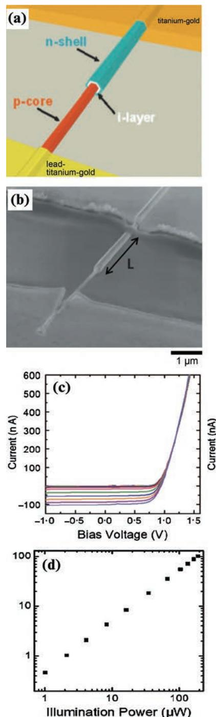
**Figure 4.** (a) Schematic view of the p-i-n structured GaAs nanowires radial photovoltaic (PV); (b) scanning electron microscope image of the corresponding PV structure; (c, d) I-V characteristics of GaAs radial PV cell under different illumination intensities from 1–200  $\mu\text{W}$ . Reprinted with permission from Colombo *et al.* (2009).
