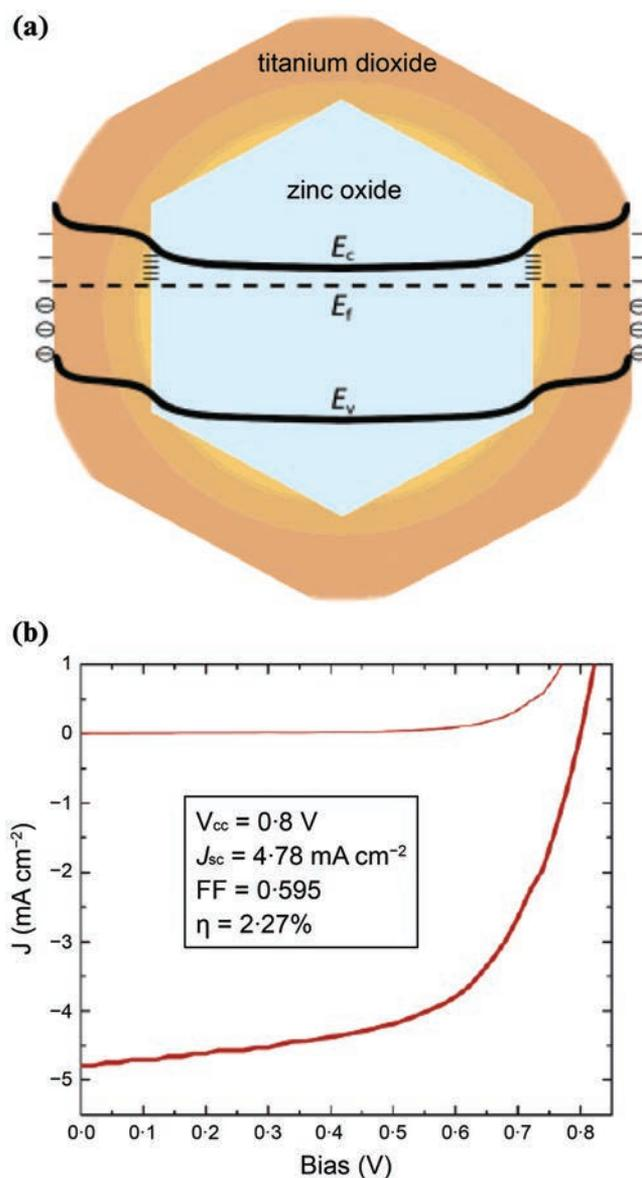
**Figure 7.** (a) Schematic energy level of zinc oxide (ZnO) core and titanium oxide ( $\text{TiO}_2$ ) shell; and (b) I–V characteristics of PV cell based on ZnO– $\text{TiO}_2$  core-shell structure. Reprinted with permission from Law *et al.* (2006).
