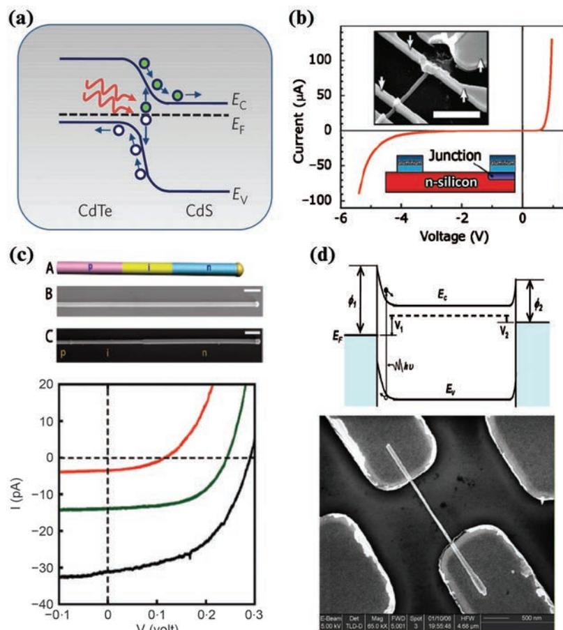
**Figure 3.** (a) Schematic view of the photovoltaic (PV) mechanism; (b) PVs based on metal-semiconductor Schottky contact; (c) PVs based on semiconductor p-n (p-i-n) junctions in single nanowire; and (d) PVs based on asymmetric contact. Reprinted with permission from Fan *et al.* (2009a, 2009b, 2009c), Kelzenberg *et al.* (2008), Kempa *et al.* (2008) and Liao *et al.* (2008).
