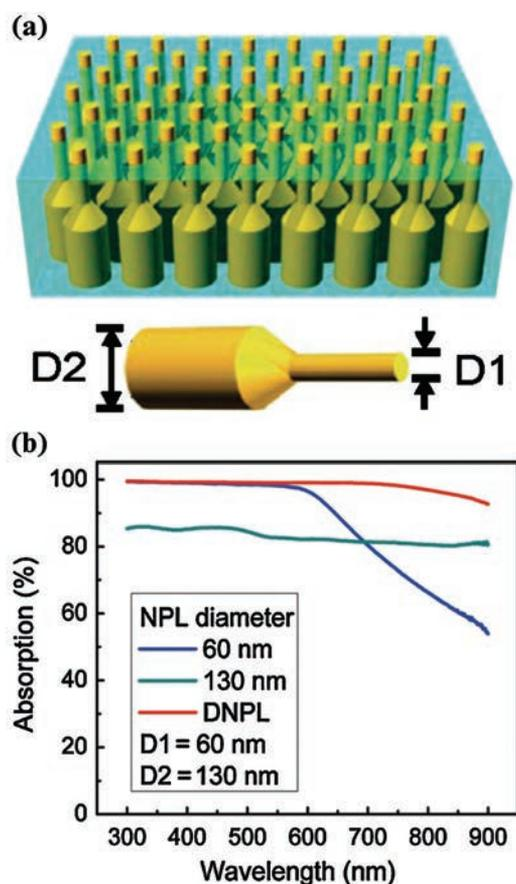
**Figure 1.** (a) Schematic diagram of the dual-diameter nanopillar array layer (DNPL); and (b) light absorbance comparison of the DNPL layer with those of uniform diameter nanopillar arrays. Reprinted with permission from Fan *et al.* (2010).
