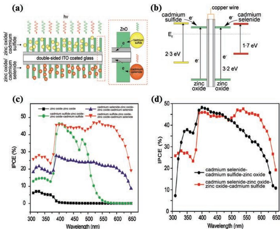
**Figure 10.** (a) Schematic view of the double-sided CdS–ZnO–ZnO–CdSe photoanode; (b) band energy alignment of the double-sided photoanode; (c) incident photon-to-current conversion efficiency (IPCE) spectra of the double-sided photoanode in the range of 310–650 nm at 0 V; and (d) IPCE comparison with single-sided CdSe–CdS–ZnO photoanode. Reprinted with permission from Wang *et al.* (2010).
