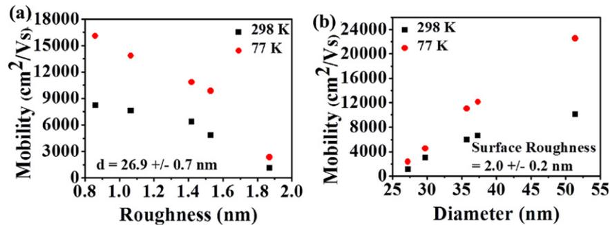
**Figure 4.** The dependency of peak field-effect mobility on (a) NW surface roughness (diameter =  $26.9 \pm 0.7$  nm) and (b) NW diameter (surface roughness =  $2.0 \pm 0.2$  nm) at temperatures of 77 and 298 K.
