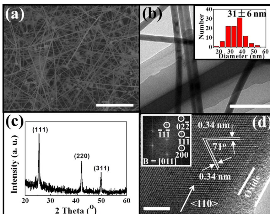
**Figure 1.** (a) SEM image of the as-obtained InAs NWs (scale bar = 2  $\mu\text{m}$ ). (b) TEM image of the NWs depicted in panel (a) (scale bar = 200 nm). The inset shows the diameter statistics of 100 NWs observed in the TEM study. (c) XRD spectrum of the grown NWs. (d) High-resolution TEM image of a representative NW shown in panel (a) (scale bar = 5 nm). The inset displays the corresponding fast Fourier transform reciprocal lattice spots where the [110] zone axis is identified.
