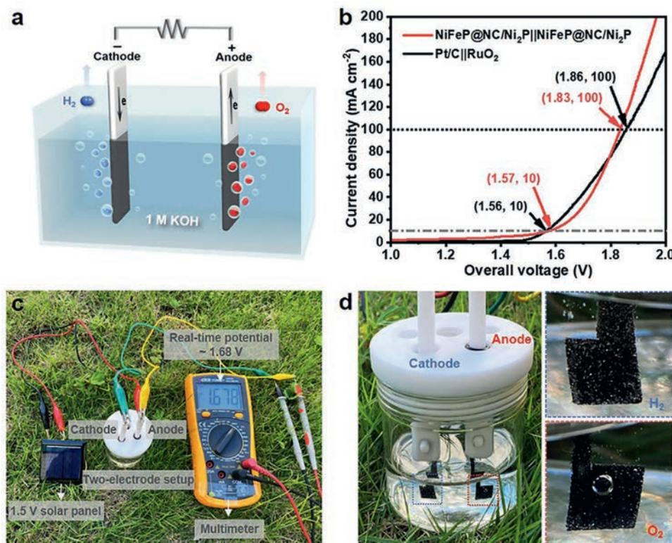
**Figure 5.** a) Schematic illustration of the two-electrode setup for overall water splitting. b) Polarization curves of NiFeP@NC/Ni<sub>2</sub>P||NiFeP@NC/Ni<sub>2</sub>P and Pt/C||RuO<sub>2</sub> in a two-electrode configuration for water splitting. c) Digital photograph of the NiFeP@NC/Ni<sub>2</sub>P||NiFeP@NC/Ni<sub>2</sub>P couple driven by a solar cell. d) Magnified photograph of the two-electrode setup and the electrodes.
